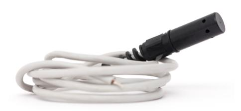
The **Sen-Humi** sensor probe is based on SHT21 digital temperature and humidity chip. It consists of **ABS cover** and **1 meter cable** with four (4) internal wires. Provides 8-bit to 12-Bit% RH relative humidity and 12-bit to 14-bit Celsius temperature measurements. The **Sen-Humi** communicates over a **I**<sup>2</sup>**C interface** that requires two (2) data lines for communication with a central microprocessor. In addition, the **Sen-Humi** is fully calibrated.
