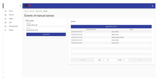
**Figure 14:** Sensor's Events page. At this page the user can view the events history of the sensor. By picking up the dates he wants, events like connectivity status or "wake up button pressed" will appear.
