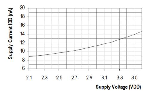
**Figure 7** Typical dependency of supply current (sleep mode) versus supply voltage at 25°C. Please note that deviations may be up to ±50% of displayed value. Values at 60°C scale with a factor of about 15 (compare Table 1).
