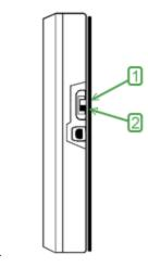
Figure 5 (Power Switch 1:Off, 2:On)
