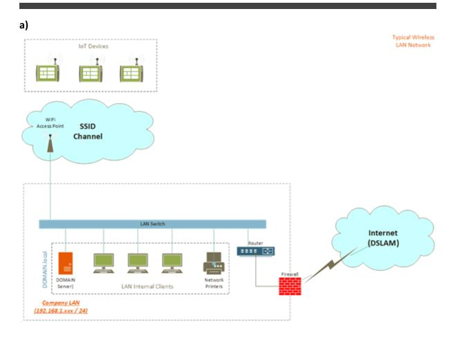
Using the implementation above, IoT devices connect directly to a Wireless Access Point, which is in Bridge Mode with the Main Network
