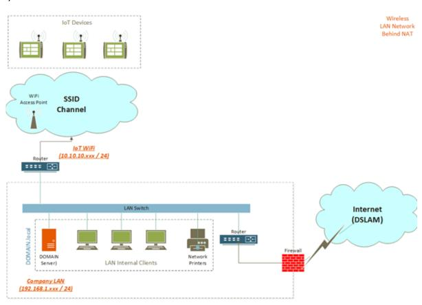
Using the implementation above, IoT devices connect directly to a Wireless Access Point, which is in Bridge Mode with a secondary Router, which is in NAT Mode to the Main Network
