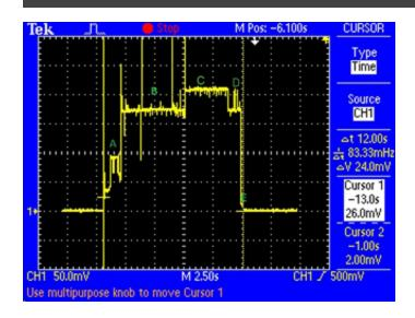
In this waveform we can see all the stages of the device from wake up to sleep again.
